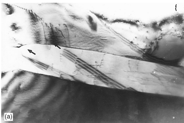
Figure 2 Degenerate \alpha_1 plate (623 K, 1200 s).
